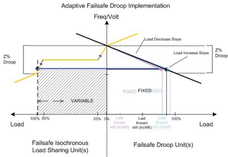
Figure 1. Failsafe Adaptive Droop Operation adapts over time as the load changes to stabilize the system.
