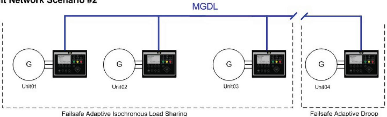
*Scenario 1. If a controller (Unit 01, for example) detects fewer than half the expected number of controls online (a minority), then the minority operate in the Failsafe Adaptive Droop mode and the balance in the Failsafe Adaptive Isochronous Load Sharing mode.*
