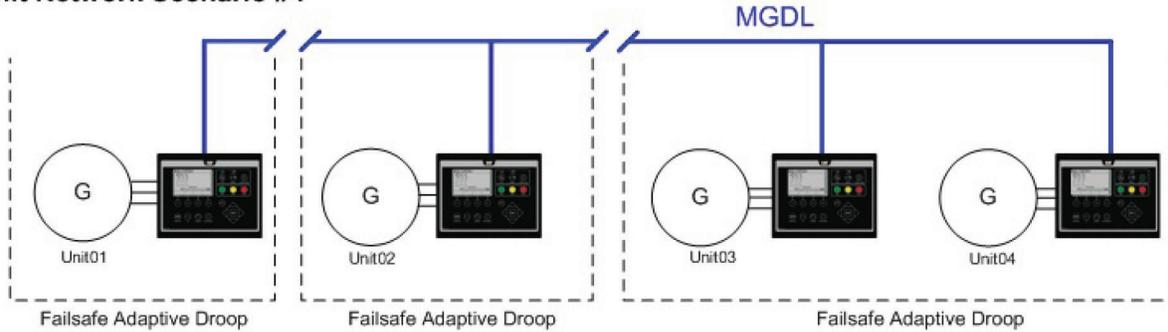
*Scenario 3. If a controller detects exactly half the expected number of controls on the network, there are two possibilities. If the control detects the lowest unit number, then that unit and the other units in its half operate in Failsafe Adaptive Isochronous Load Sharing mode, and the other half operate in the Failsafe Adaptive Droop mode. If the control does not detect the lowest unit number, the opposite occurs.*
