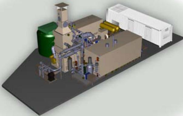
The base hybrid configuration is a 1 MW fuel cell plus a 2 MW gas generator set, both using natural gas fuel. The fuel cell provides 1 MW of baseload generation, and the gas generator set provides 2 MW of peaking capacity, for a total of 3 MW. Any number of
