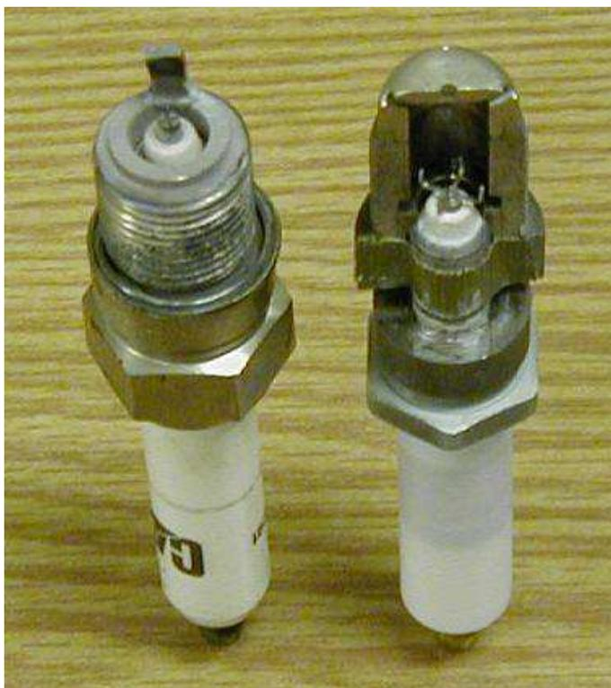
*Figure 4: J-gap (left) and prechamber (right) spark plugs*
