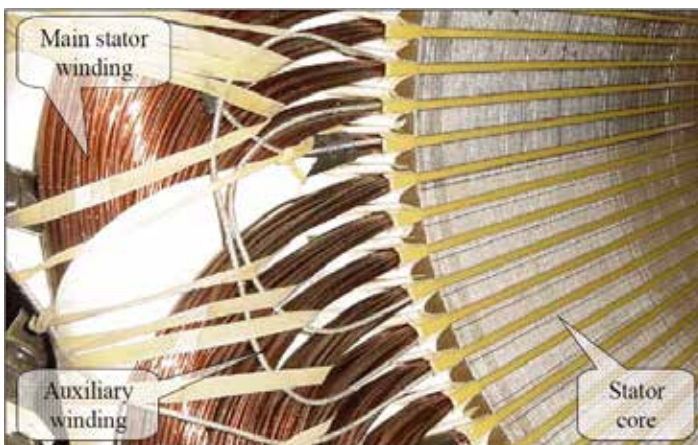
Figure 1. IE Low Voltage Stator Winding
