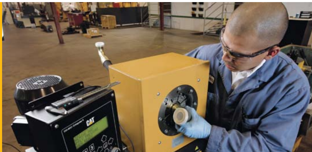
Cat Dealers pneumatically clean hoses with foam projectiles to remove contaminants that can damage hydraulic system components.
