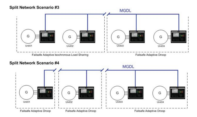
Scenario 3. If a controller detects exactly half the expected number of controls on the network, there are two possibilities. If the control detects the lowest unit number, then that unit and the other units in its half operate in Failsafe Adaptive Isochronous Load Sharing mode, and the other half operate in the Failsafe Adaptive Droop mode. If the control does not detect the lowest unit number, the opposite occurs.
