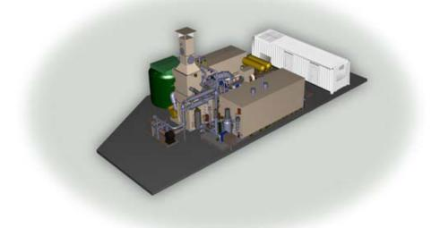
The base hybrid configuration is a 1 MW fuel cell plus a 2 MW gas generator set, both using natural gas fuel. The fuel cell provides 1 MW of baseload generation, and the gas generator set provides 2 MW of peaking capacity, for a total of 3 MW. Any number of
