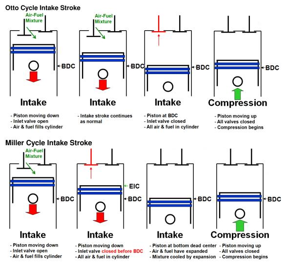
Figure 7: Intake stroke for an Otto Cycle engine (above) and a Miller Cycle engine (below)
