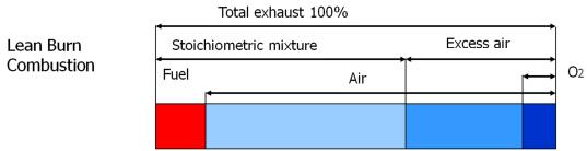
Figure 12: Lean burn combustion air/fuel ratio
