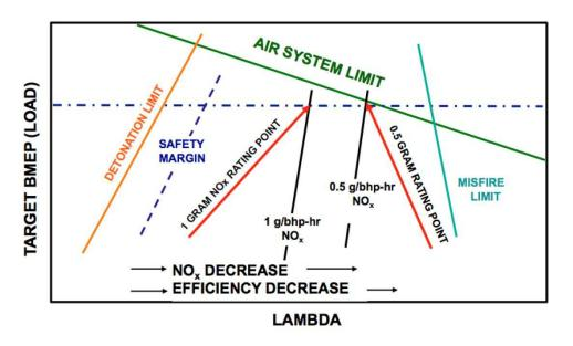
Figure 3: Lean burn gas engine rating limits
