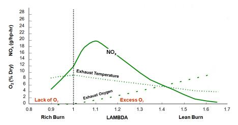
Figure 13: Typical LAMBDA vs. NO<sub>x</sub> emissions map
