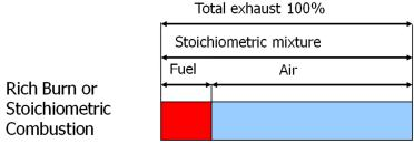
Figure 11: Rich burn (stoichiometric) combustion air/fuel ratio
