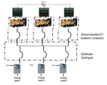
Figure 1: Sample single line of a Cat<sup>®</sup> EMCP 4.4 On-board Paralleling system featuring genset mounted electrically operated circuit breakers with prioritized load shed/add capability.
